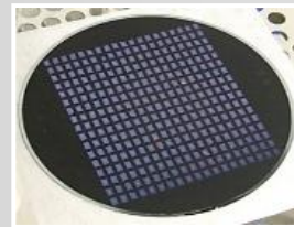
FO-WLP die first, RDL first, multi-strata, organic, silicon, glass substrates
