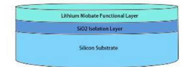
Structure of a Lithium Niobate Thin Film with Silicon Substrate and SiO 2 Isolation Layer
