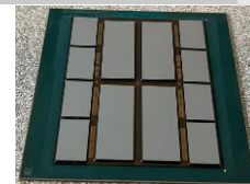
Large (~3x reticle size) fan-out package for chiplet integration
