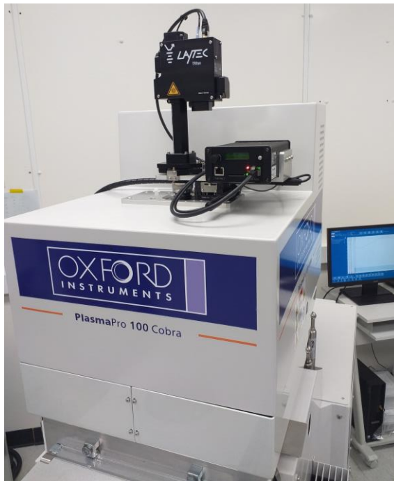
Fully-integrated LayTec EPD with Oxford Instruments PP100 Cobra ALE system
