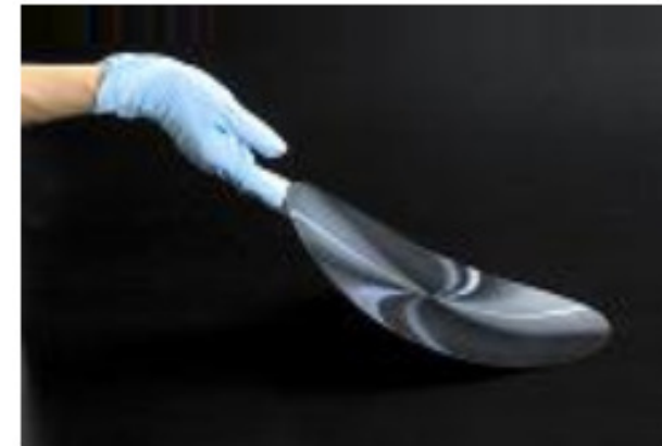
Photo 5: t50 μm Φ8-Inch Silicon Wafer
