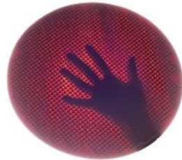
Photo 1: t5 μm, Φ300 mm Silicon Wafer(Supplied by Renesas Technology Corp)
