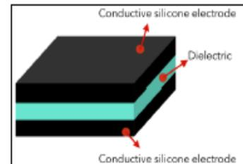
Figure 1(a): Schematic of *Compo-SiL*<sup>®</sup> (b) *Compo-SiL*<sup>®</sup> E Series
